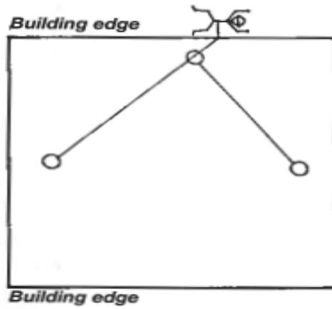
*Use of a secondary anchorage and lanyard or lifeline removes or reduces the pendulum effect*
